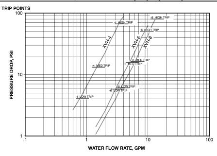
Note: XVH-4 is inlet/outlet size of 1/4" XVH-6 is inlet/outlet size of 3/8", 6mm XVH-8 is inlet/outlet size of 1/2", 8mm
