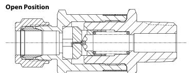
The spring holds the poppet in the open position during normal flow. When flow increases to the predetermined rate or trip point, the poppet will close.
